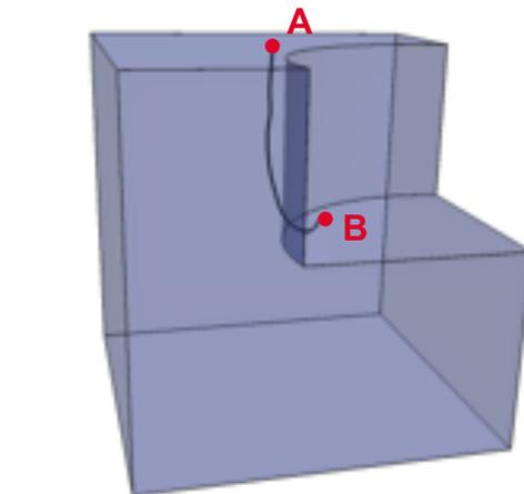
Singularity line in the generated frame field
